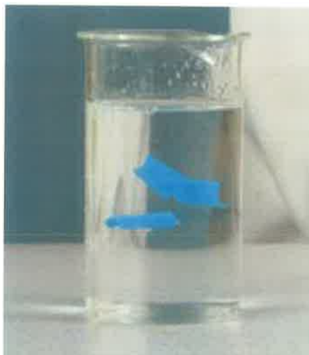
At this point, the densities of the plastic and the solution are the same.
