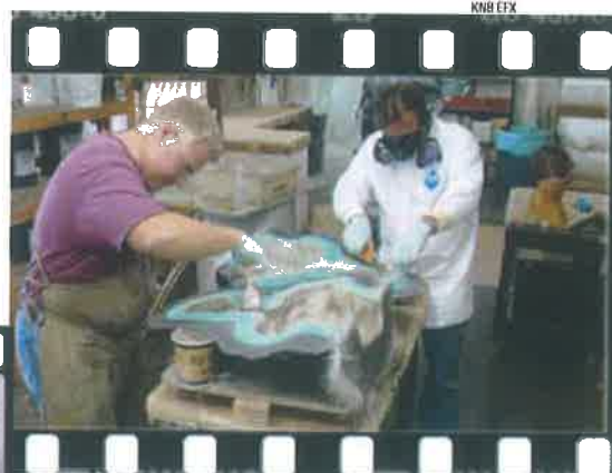
Two mold makers from KNB EFX fill a silicone mold with fiberglass to make a life cast for an actor. Wrinkled skin or bite marks will be sculpted on this cast later.
