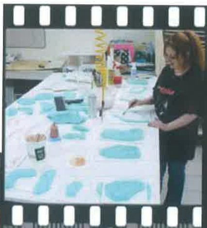
An employee of KNB EFX prepares molds that will be filled with silicone. Once the silicone sets, it is peeled from the molds and glued to an actor's face.
