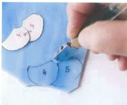
Figure 2. The artist first draws patterns on paper and then reproduces them on the glass before cutting the pieces of glass.
