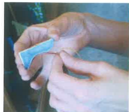
Figure 3. Each piece of glass is wrapped with copper foil because solder adheres to metal but not to glass.
